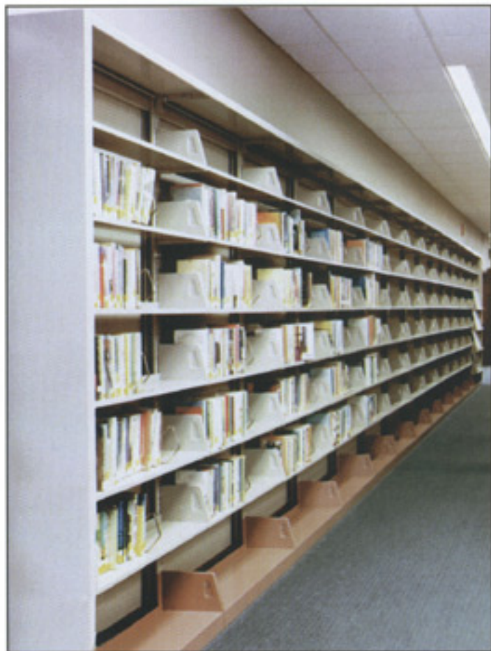
Adjustable integral backstop shelves with sliding book supports.
