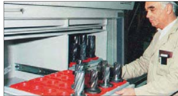
Hanel tool carrier system
