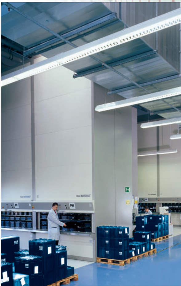
Antistatic storage in the production hall
