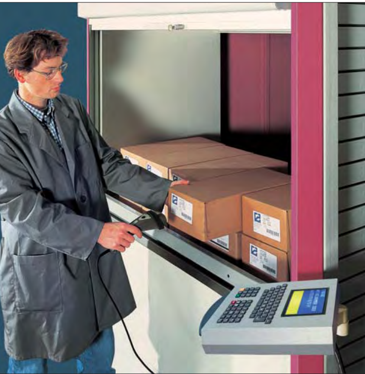
Lean-Lift from Hanel with automatic feed. The control keyboard is fixed on the container guide rails
